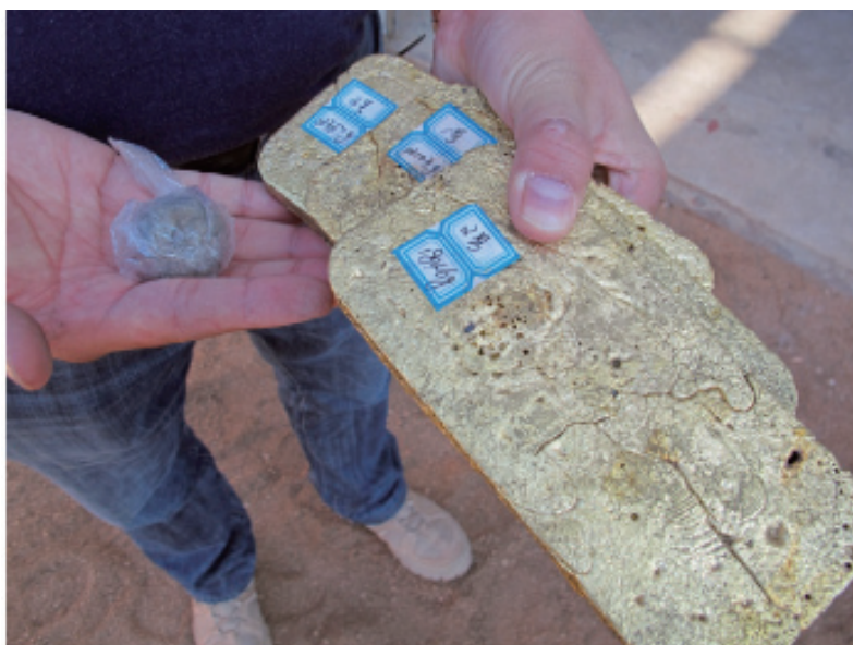
Figure 1 – Dore Gold Bars (right) produced from physical gold amalgam at Aohanqi Plant
